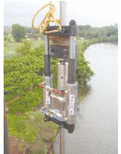
Threaded Bar Tensioning And Mechanical Locking System For Suspension Bridge (Capacity 20t, Stroke 200 mm)
