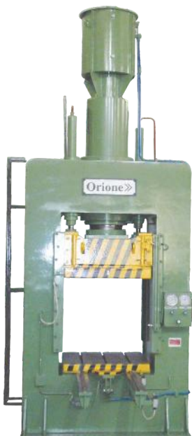
250 ton Semi-Automatic Moulding Press (Hydraulic table travel, Electrically heated platen)
