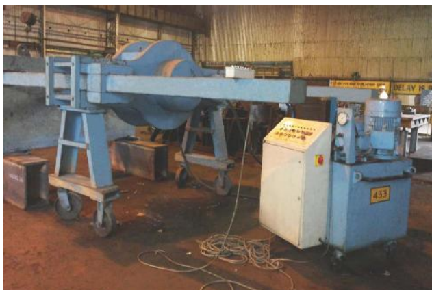
400 ton Horizontal Press (Steel plant - shaft dismounting)
