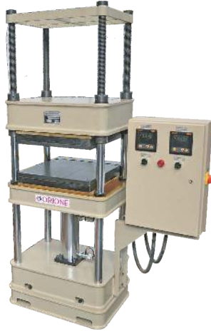
20 ton Lab Press (Electrically heated platen)
