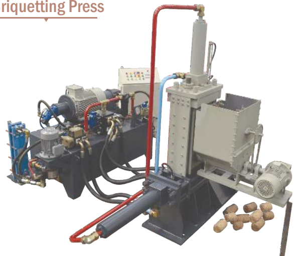
For compressing shredded garden waste into briquets of 1kg
