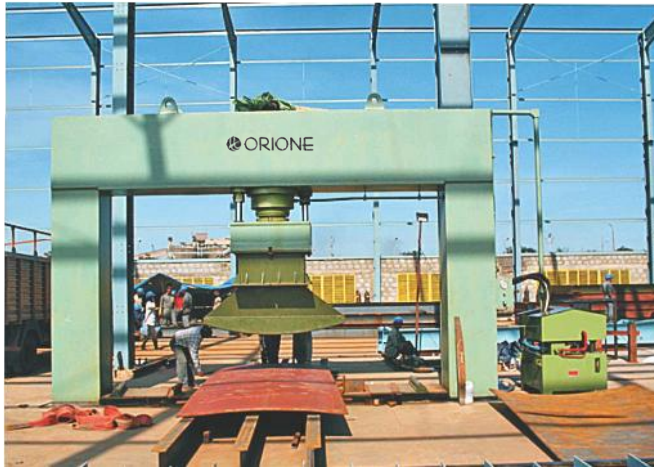
500 ton Metal Forming Press (Ship building industry)
