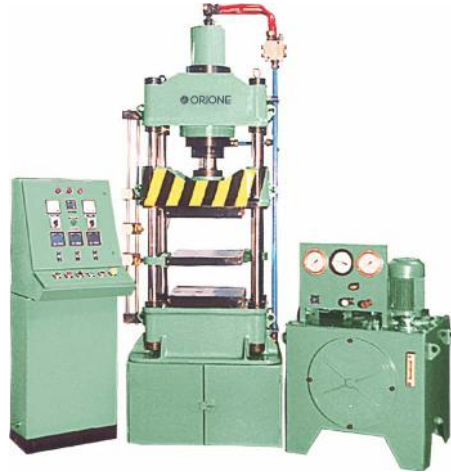
50 ton Semi Automatic Double Daylight Press (Electrically heated platen)
