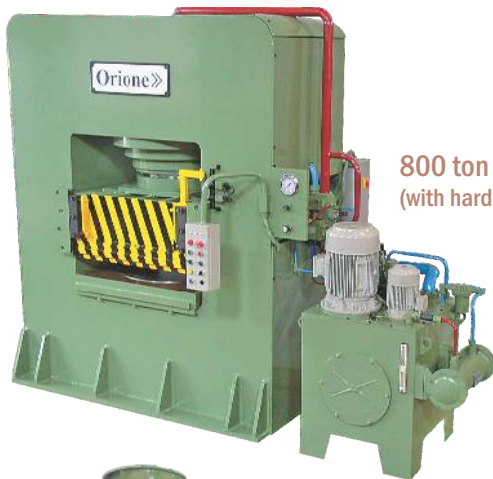
500 ton Metal Forming Press (Ship building industry)
