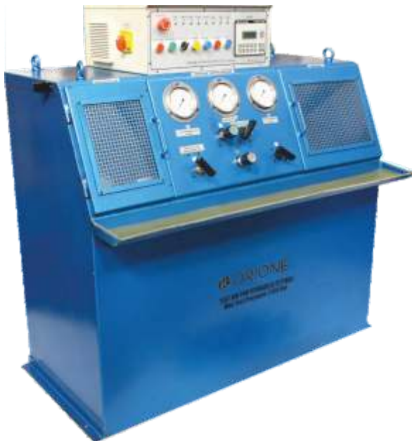
Test Rig for Hydraulic Fittings, 12-38 mm OD Max. Working Pressure 2800 bar, PLC Control
